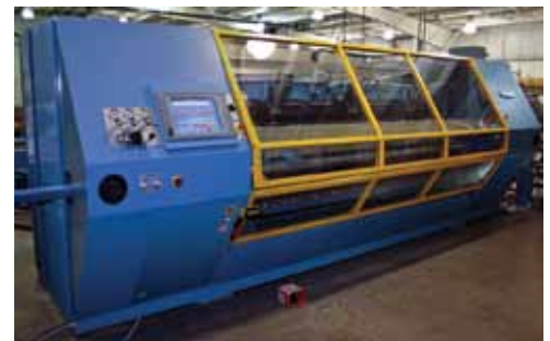
Jennerjahn JLS-120, a popular 120" wide format slitter rewinder, capable of producing 400-foot rolls in less than 30 seconds, was customized using a total package of Siemens controls and software. The robust frame on this machine makes it ideal for construction grade materials, such as house wrap, roofing and flooring underlayment, billboard vinyl and landscaping rolls.
